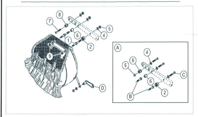
FLSTC and FLSTS Docking Hardware with Saddlebag Supports
